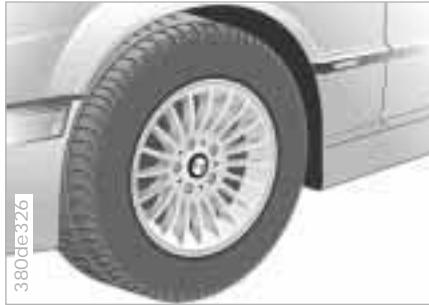
The BMW emergency run-flat tyre system with integral support ring enables the car to continue moving if pressure is lost suddenly from the tyre.
