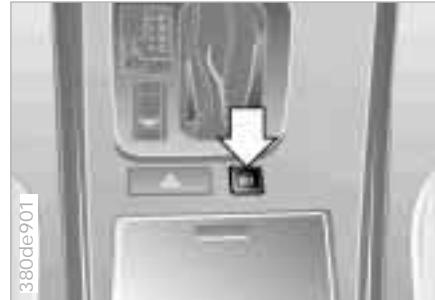
When the car is driven away from a standstill, the central locking system takes effect when it reaches a speed of 8 km/h (app. 5 mph). In an emergency, however, it can always be released manually at the central locking button (arrow) or at an inside door handle.
