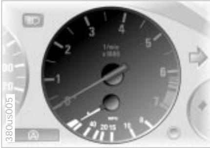
Indicates current fuel consumption in mpg (in liters per 100 km on Canadian vehicles). This instrument clearly shows whether your current driving style is conducive to economy and minimum exhaust emissions.
