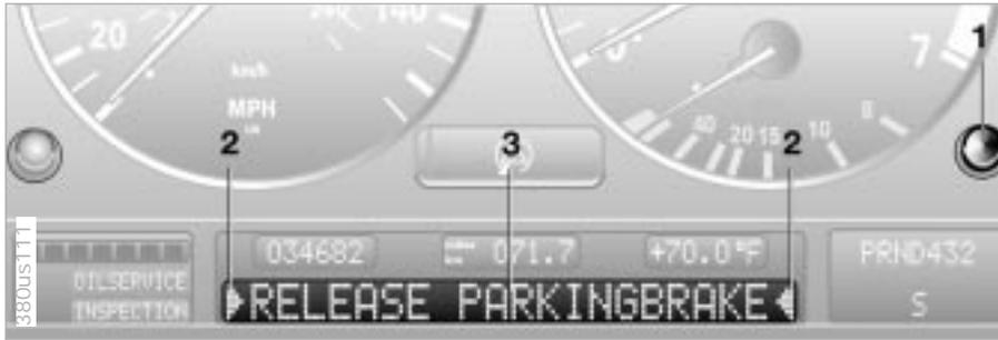
System malfunctions are reported in text form and alerts or warnings are each reported by a gong when the ignition key is in position 2.
