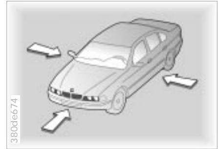
The illustration depicts schematically the primary directions of vehicle impact which initiate an airbag deployment.
