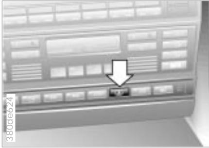
To actuate, press the button briefly with the ignition key position 1 and higher.
