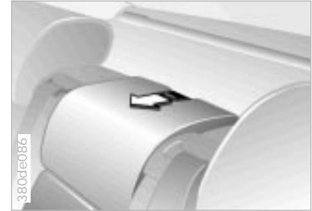
Stored between the rear seats. Pull the lever (arrow) and fold the cover forward.
