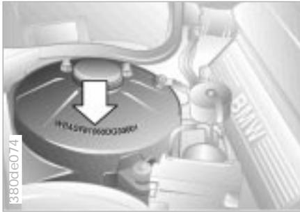
In the engine compartment, stamped on the right-hand strut dome (arrow) and on the upper edge of the instrument panel on the left side.
