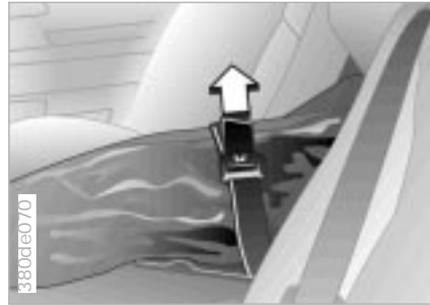
4 From the inside of the luggage compartment, use the magnetic retainers to attach the cover panel to the underside of the rear parcel tray.
