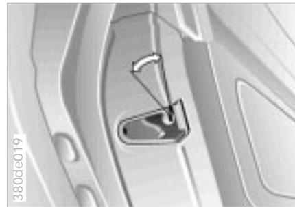
Insert the key into a rear door lock and turn it outward:
