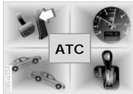
On vehicles with automatic transmission Adaptive Transmission Control (ATC) uses a number of factors to calculate the maximally efficient gear. In this process it monitors your personal driving style, the situation in which you are driving, the condition of the road and the traffic conditions.
