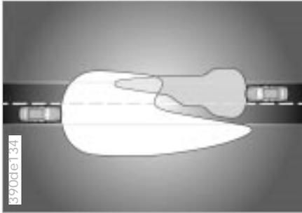
The xenon lamps light up the side and front areas of the vehicle with significantly more brightness and uniformity than the traditional halogen lamp.
