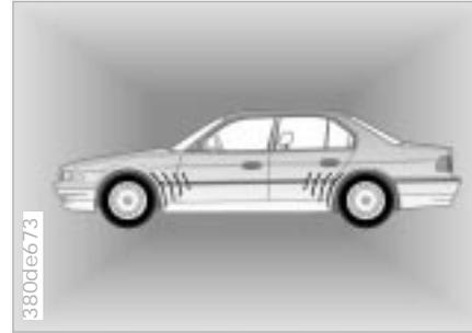
The Tire Pressure Control system assumes the task of regular tire pressure checks for you. Tire pressures are monitored at all four wheels, even when the vehicle is moving.
