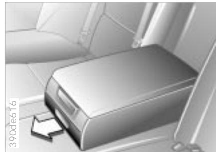
Two beverage holders are provided in the lower section of the center armrest. Pull the handle outward to open (arrow).
