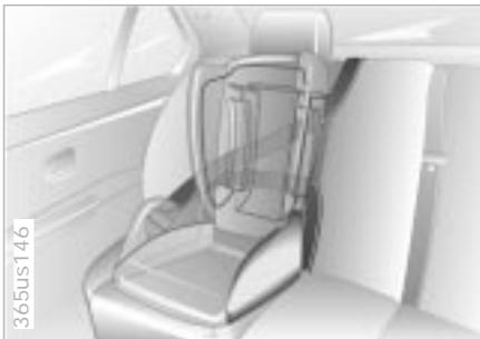
All of the rear belt retractors and the front passenger's safety belt can be locked for mounting and securing child restraint systems.
