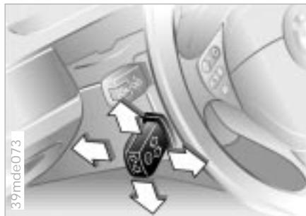
The steering wheel can be moved in any of four directions. Adjust by moving the control lever in the desired direction.
