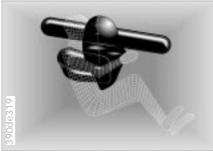
Deceleration sensors continuously monitor the physical forces acting upon the vehicle. If, as the result of a frontal collision, a deceleration is reached at which the protection of the safety belts alone is no longer adequate, the gas generators of the driver and passenger-front airbags are ignited. However, the passenger-side airbag is only triggered if an additional sensor has recognized that the passenger seat is occupied.
