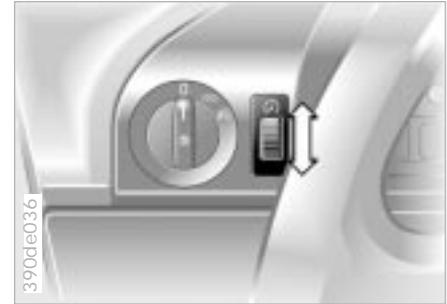
Turn the rotary dial to adjust the lighting intensity.
