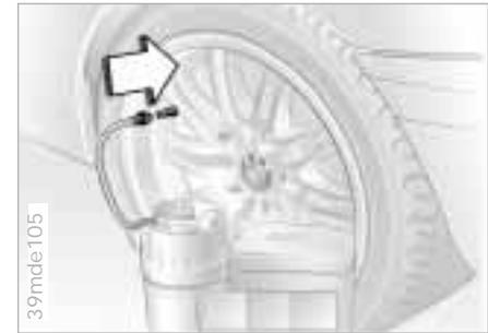
2 Take off the round cover and take out hose 4. Unscrew the valve from the defective wheel and screw the hose to the valve.
