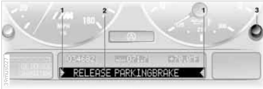
Text messages are used to alert the driver to system malfunctions with the ignition key in position 2 and higher. The alert is accompanied by a gong.
