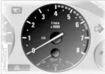
The orange early warning zone appears depending upon the engine temperature. As the engine temperature increases, more and more sectors of this early warning zone disappear.
