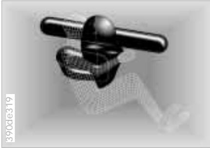
Deceleration sensors continuously monitor the physical forces acting upon the vehicle. If, as the result of a frontal collision, a deceleration is reached at which the protection of the safety belts alone is no longer adequate, the gas generators of the front airbag will be simultaneously ignited on both the driver and passenger sides. However, the front airbag on the passenger-side is only triggered if an additional sensor has recognized that the passenger seat is occupied.
