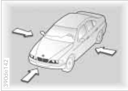
The illustration schematically depicts the primary directions of vehicle impact that initiate an airbag deployment.
