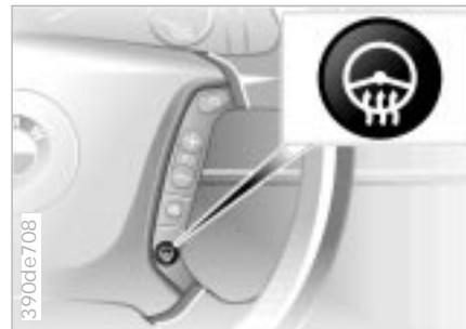
The heated steering wheel feature is available for operation when the ignition key is in position 2.
