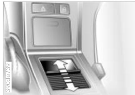
The cover of the storage compartment on the vertical surface of the center console can be pushed open or closed (illustration). If your vehicle is equipped with a cassette holder\*, open each cassette compartment by pressing on the small button.
