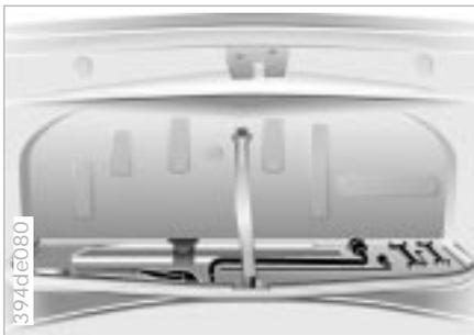
Attached to the underside of the luggage compartment lid/tailgate. Unscrew the wingnut for access.
