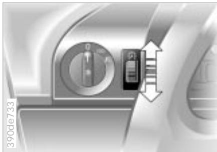
Turn the rotary dial to adjust the illumination intensity.
