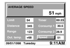
You can obtain a display of the car's average speed. The average speed is calculated for the time during which the engine is running.
