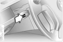
With the ignition key in position 1 and up, you can use the button in the turn signal lever to call up information from the onboard computer for display in the instrument cluster.
