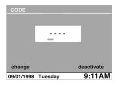
You can establish a code which will prevent the engine from being started if the code is not entered. When you have activated this code, you will be prompted to enter it at ignition key position 1.
