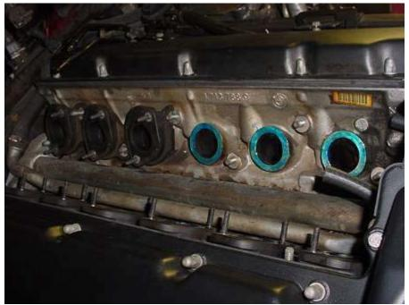
•TOP: Here is the manifold gaskets installed; note that there is Hylomar on the front gasket.
