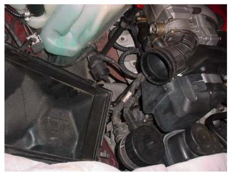
TOP: Left MAF, with electrical plug still in place, and air filter top in place.
