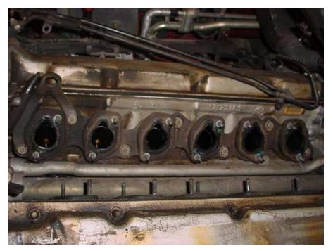
BOTTOM: This is the left side showing the intake manifold gaskets. Not the engine pulling bracket at the back on this side.
