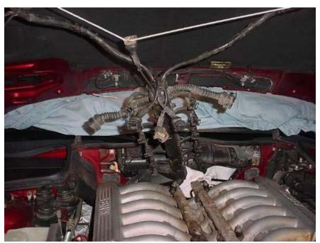
TOP: This is the fuel injector rails with the fuel injector still in place, after the wire housing as been removed.
