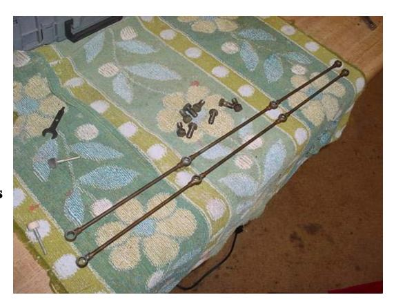
TOP: As you can see, the bottom pipe shows the holes that are between the banjo bolts. Make sure all these holes are cleaned out before putting them back on.
