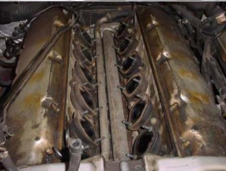
TOP: This is the right side showing the intake manifold gaskets. Note the engine pulling bracket at the front on this side. The two pipes are the return fuel lines that go from the front of the fuel rails to the back of the engine.
