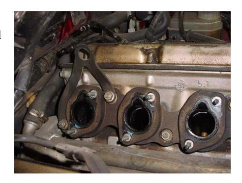
TOP: This is the right cylinder head with the intake gaskets removed.
