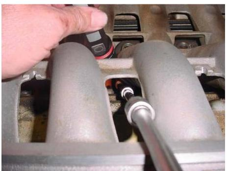
TOP: This is 1 of 4 nuts that hold the intake manifold on to the 4 holders located on each outside corner of the valve cover, above the spark plugs.
