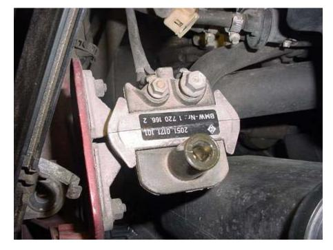
BOTTOM: Left side Coil with the wires installed. Both coil wires (big one and small one) must be removed to allow the wire harness to be moved so the intake manifold can be removed.
