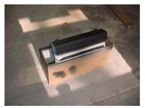
BOTTOM: This is the right intake manifold after I've polished the BMW and horizontal lines.
