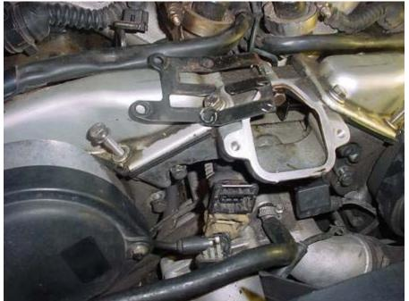
TOP: This is a view of the left side Pulse Sender (top) and Cylinder Identifier 7 through 12 (bottom) with the bolts taken out.
