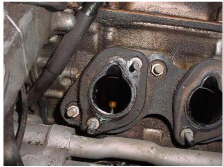
This is the rear engine pulling bracket; it is located on the left side. It is bolted to the intake manifold gasket bolt, and is held on by two 12mm nuts. Just like the front, after the bracket is removed there is another set of nuts holding the gasket on.
