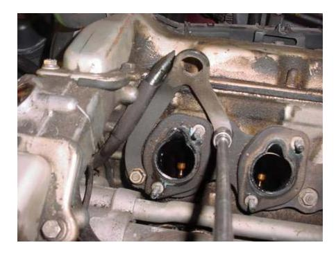
BOTTOM: After the bracket is removed there is another set of nuts holding the gasket on.
