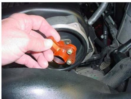
TOP: Using a 6mm Allen socket I'm taking the drive flange bolt out of the end of the camshaft.
