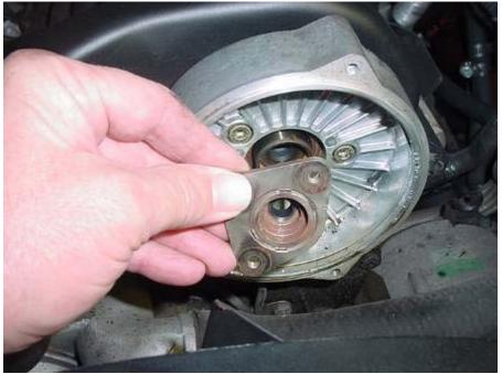
TOP: Using a 5mm Allen socket I'm taking the three bolts out of the Distributor housing.
