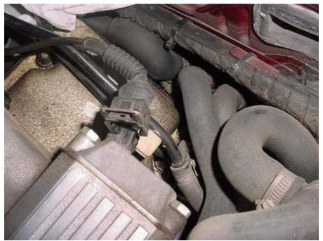
BOTTOM: This is a view of the two fuel tank breather valves. One on top has a black connector and the one on the bottom has a tan connector, don't get these mixed up!
