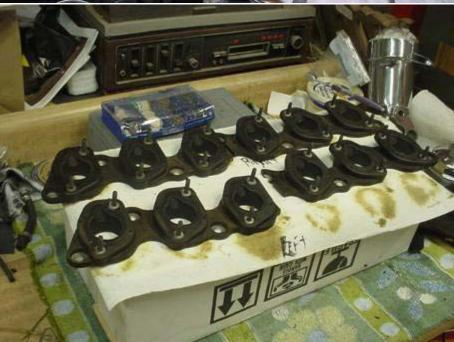
•TOP: Here are the intake ports after being cleaned and ready for the Hylomar to be installed.
