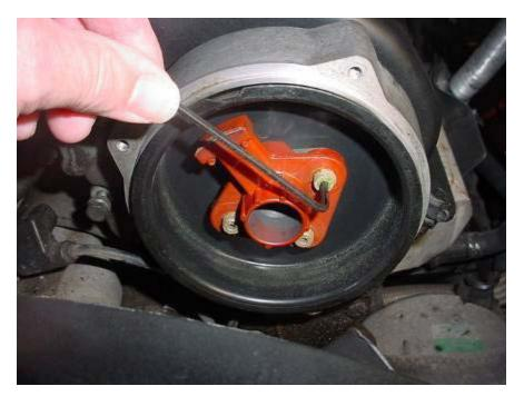
BOTTOM: I'm taking the rotor off of the drive flange
