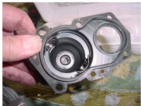
TOP: Here are the three screws that hold the brush and encoder housing on to the throttle body housing.
