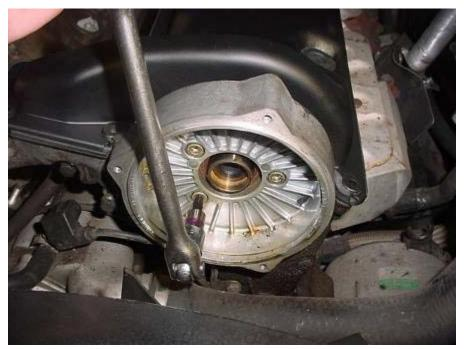
BOTTOM: I'm taking the Distributor housing off of the cylinder head.
