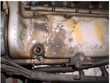
TOP: This is the front engine pulling bracket; it is located on the right side. It is bolted to the intake manifold gasket bolt, and is held on by two 12mm nuts.
