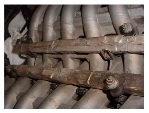
BOTTOM: This is one of four bolts (two on each side) that holds the fuel injector on the intake manifold.
