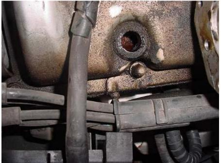
This is one of two temperature sensors located at the back of each of the intake manifold, this is the one on the left side.
