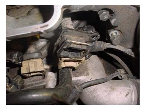
BOTTOM: This is the Pulse Sender and Cylinder Identifier removed from the clips that are used to bolt them to the Cylinder Head. Note the black clip on the top and the tan on the bottom; don't cross them.
