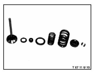
Low valve mass and dual valve springs insure reliable opening and closing between the short ignition periods.
