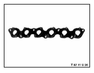
Elastic sealing plates are used to attach the plenum assemblies to the cylinder heads. This feature acts as a sound barrier and limits vibration to the electronic throttle valve assemblies.
