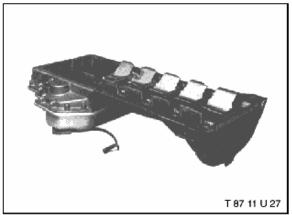
Correct hydraulic tappet operation requires engine oil which is free of all air bubbles. A special oil deflector (windage tray), located in the oil pan, defoams the oil and limits splash oil precipitation.
