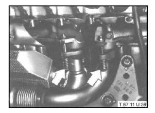
The four exhaust down pipes of the exhaust assembly are mounted with spring loaded ball flanges (arrows). This arrangement insures positive sealing and tends to release any trapped stress.
