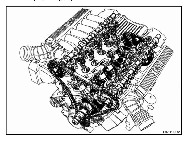
This valve arrangement in conjunction with the piston bowl forms a compact combustion chamber with excellent cylinder filling and evacuating characteristics.
