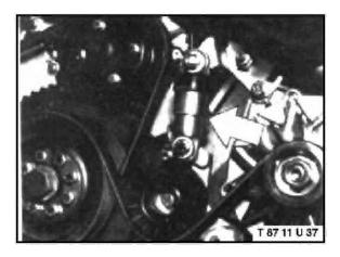
All accessory component rotary drive is accomplished with two poly-V type drive belts. Once correctly installed the belts are self-adjusting with automatic hydraulic tensioners (arrow) and thus are maintenance-free.
