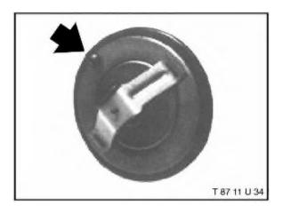
Cooling system flow to the radiator is regulated with an 800 C thermostat. A ball type valve (arrow) in the thermostat plate allows air bubble bleeding following cooling system service.
