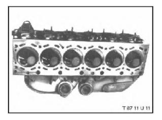
Cylinder heads are manufactured of die cast aluminum and are identical for both banks.
