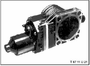
Each intake plenum chamber is equipped with a fast acting, electronic throttle valve assembly.
