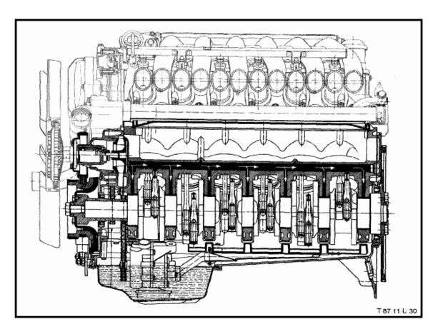
Lubrication oil routing - Camshaft, crankshaft and connecting rods
