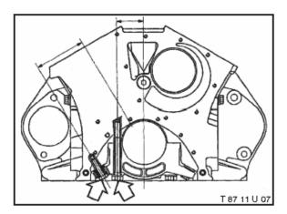
The lightweight aluminum crankcase is manufactured hypereutectically. That is to say, special measures are employed during the formation, casting and cooling which promote torsional resistance and dimensional stability.
