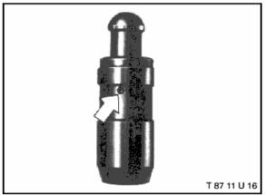
The operation of the self-adjusting valve clearance system is based on engine oil pressure hydraulics. Clearances are taken up as oil pressure enters the hydraulic tappet through the oil feed bore (**arrow**) and internal one-way valve. The hydraulic pressure acts on the adjusting piston which is displaced to reduce any nonspecified clearance.
